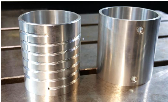
Cylindrical Liquid Cold Plate
